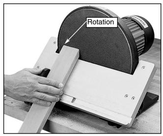
Figure 10. Mitering with table angled.
